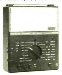
selection, single rotary switch for range selection and V-ohm on the same input sockets.
