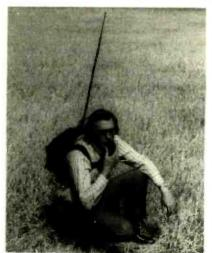
"MANPACK" COMBAT RADIO HAS 280,000 channels to select from. Using groundwave transmission for distances of a few thousand yards and skywave transmission for possible ranges in the thousands of miles, it will normally be used for distances ranging from local up to a few hundred miles.
